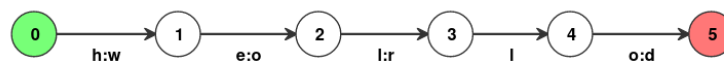
Figure 7: In Jupyter cell #4, an empty FST is first constructed using FST() with the default semiring. The edges are added one at a time using add_arc , where most edges have different labels on the input and output side.
